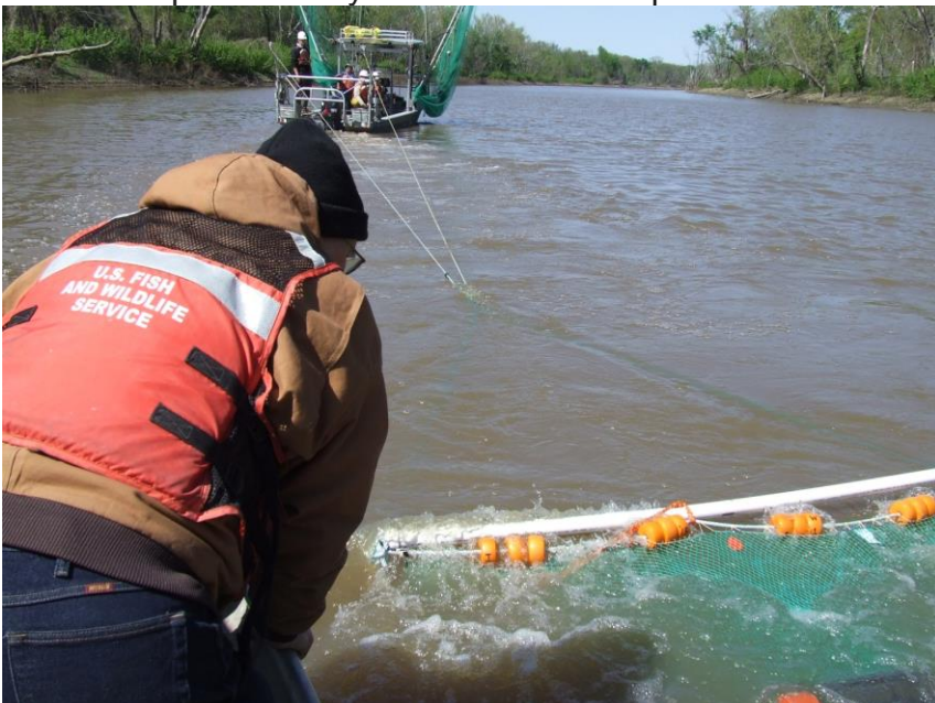
Caption: Greg Faulkner, netmaker with Innovative Nets, evaluates experimental 7' trawl net attached to a PVC frame and towed behind a boat on a tributary of the Missouri River.
