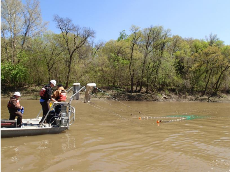
Caption: Surface trawl with experimental aluminum doors being deployed off the back of a boat.
