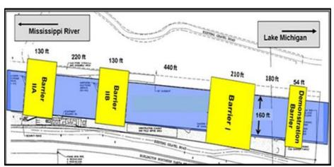
Figure 7. USACE Electrical Dispersal Barrier System.
