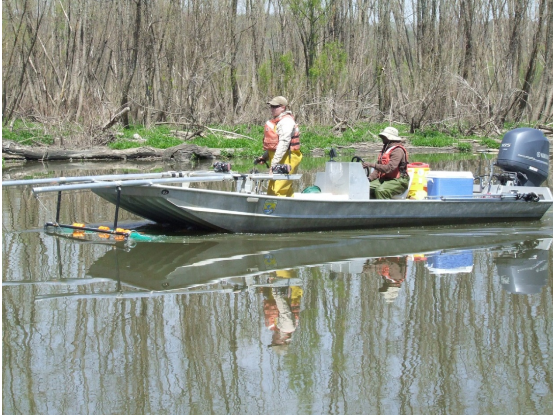
Caption: The dozer trawl in action on Lake Depue. The net can also be attached to a rigid frame and towed.
