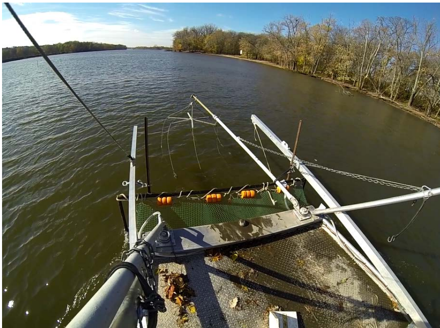
Image 1. The electrified dozer trawl with the electrified boom out front and the dozer frame behind where the fish are scooped up and held in the net.
