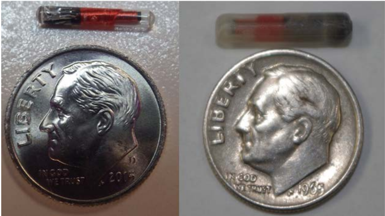
Figure 1. Images of both the PIT tag (left) and JSATS acoustic tag (right) used in the retention and mortality pilot study of juvenile Silver carp.
