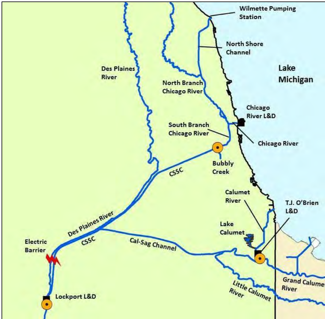
Figure 2. Map of the Chicago Area Waterways System (CAWS), showing the location of navigation dams, the electric barrier on the Chicago Sanitary and Ship Canal (CSSC), and sites sampled as part of this study. Navigation dams are represented by squares; sampling sites are represented by circles.
